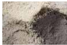
Fly ash ranges in color from gray to buff depending on the type of coal.
