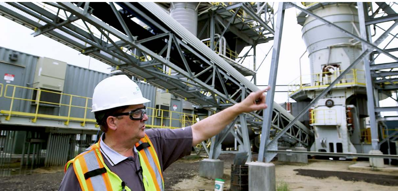
Eco's bottom ash grinding facility in central Texas processes bottom ash for sale into concrete markets.
