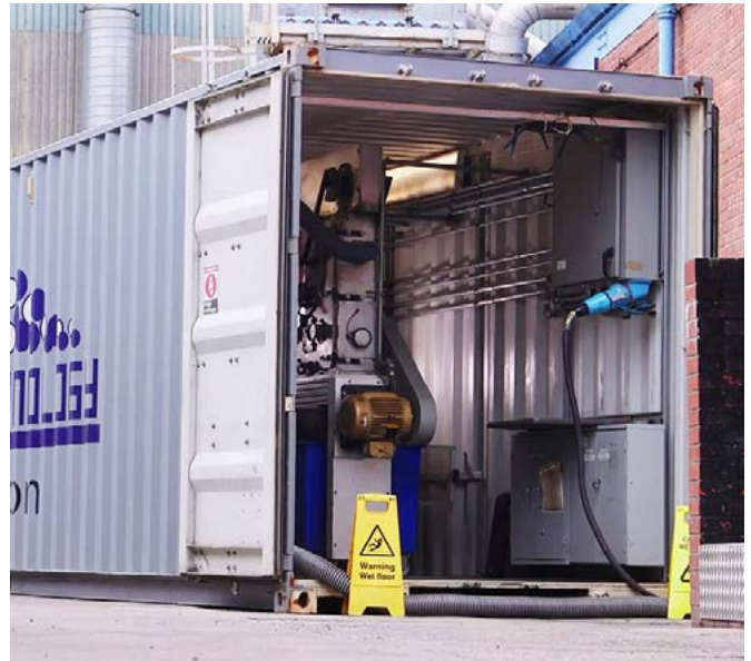
STET's triboelectrostatic separator, which can process up to 40 tons of material per hour.
