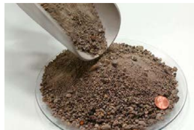
Bottom ash is a granular material suitable for replacing gravel and sand.
